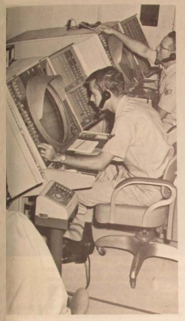
imulation team members direct their interceptors ward approaching enemy aircraft during a simulated ussion. By using switch actions, the "intercept pits" are able to guide their aircraft to the target.
