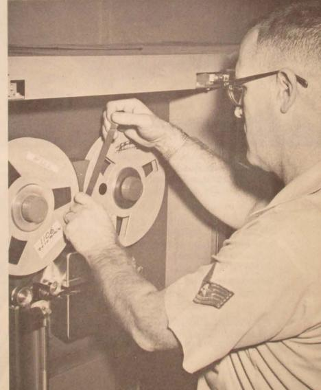
A member of a SAGE computer section loads a tape that will feed simulated flights and situations into a computer, allowing practice intercepts without actual flights.
